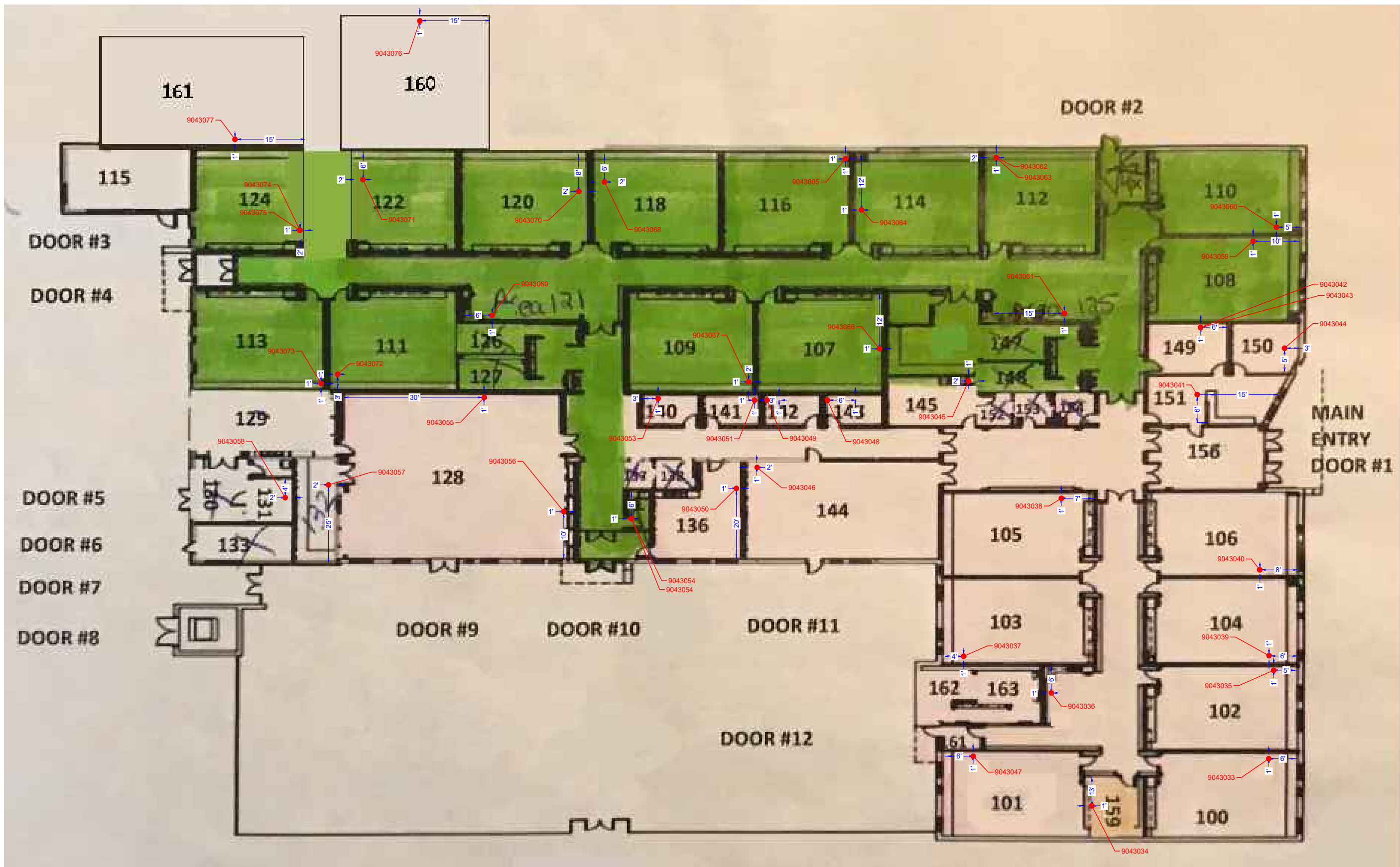
1 RADON SAMPLE LOCATIONS GROUND FLOOR PARTIAL PLAN NOT TO SCALE
