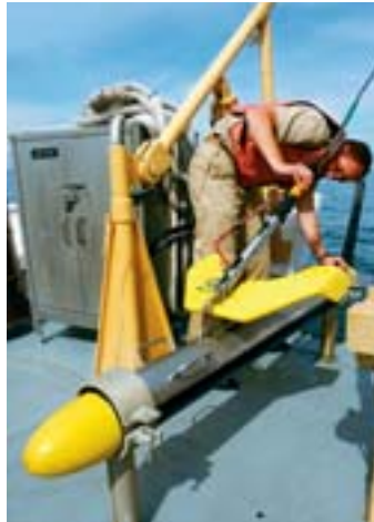
A fish-shaped sonar instrument can search for objects on the ocean floor.
